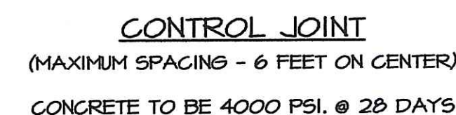
SIDEWALK DETAIL NOT TO SCALE
